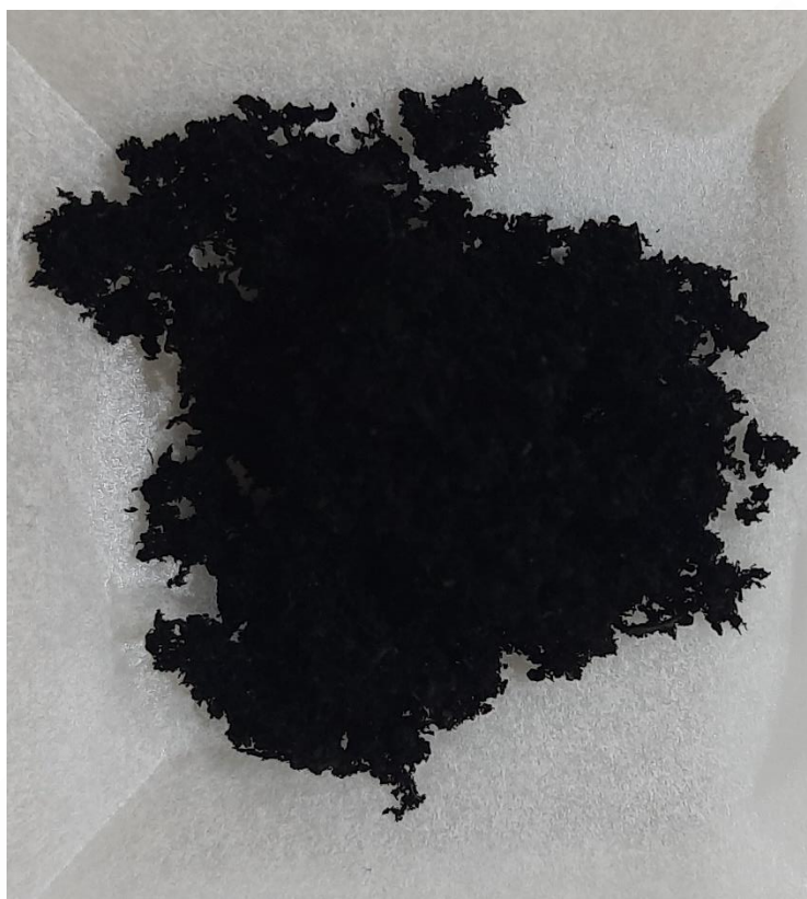
Figure: Physical Appearance of purified NoPo HiPCO SWCNT ( Produced in July 2021 )
